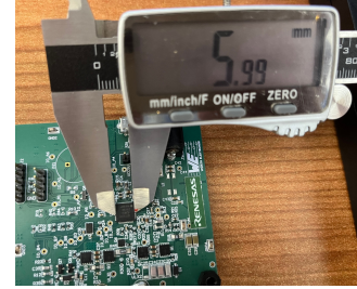
Figure 20: Microcontroller chip on the wireless charger
